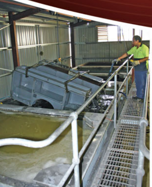
5-Stage Full Immersion Zinc Phosphate Coating System.
