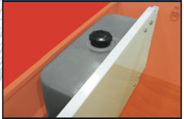
Water Tank - Polyethylene - 29lt apron mount - (tap in tail light)
